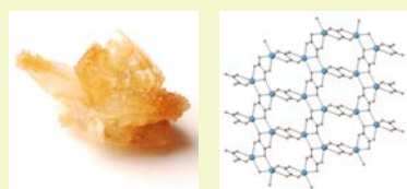
Fig. 1. (left) Photo of a macroscopic crystal of calcium oxalate and (right) its microscopic crystal structure determined by single-crystal X-ray diffraction analysis.
