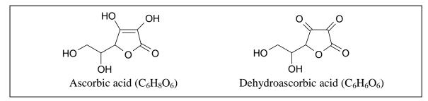
A typical titrant used for the redox titration of ascorbic acid is potassium iodate, KIO<sub>3</sub>. If the titration is carried out in 1 M HCl medium, then the reaction proceeds as follows:
