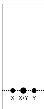
Fig. 1.1 Spots on the TLC plate before development; X: 1,4-DHP, Y: Reaction mixture.
