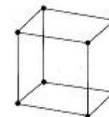
4.8 The primitive cubic unit cell and its lattice-point representation.
